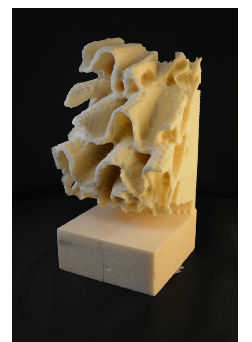
A ShopBox 5-axis mill (left) was used to machine a foam model (right) from CT data, using an ASDF instead of a mesh as an intermediate representation.
