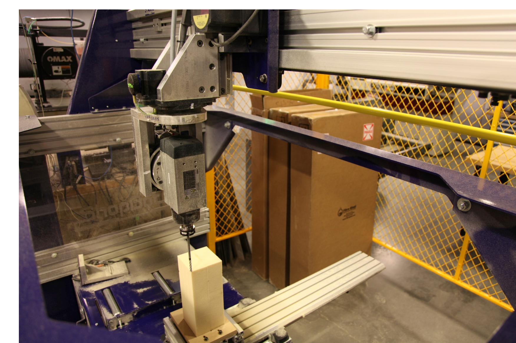
A ShopBox 5-axis mill (left) was used to machine a foam model (right) from CT data, using an ASDF instead of a mesh as an intermediate representation.
