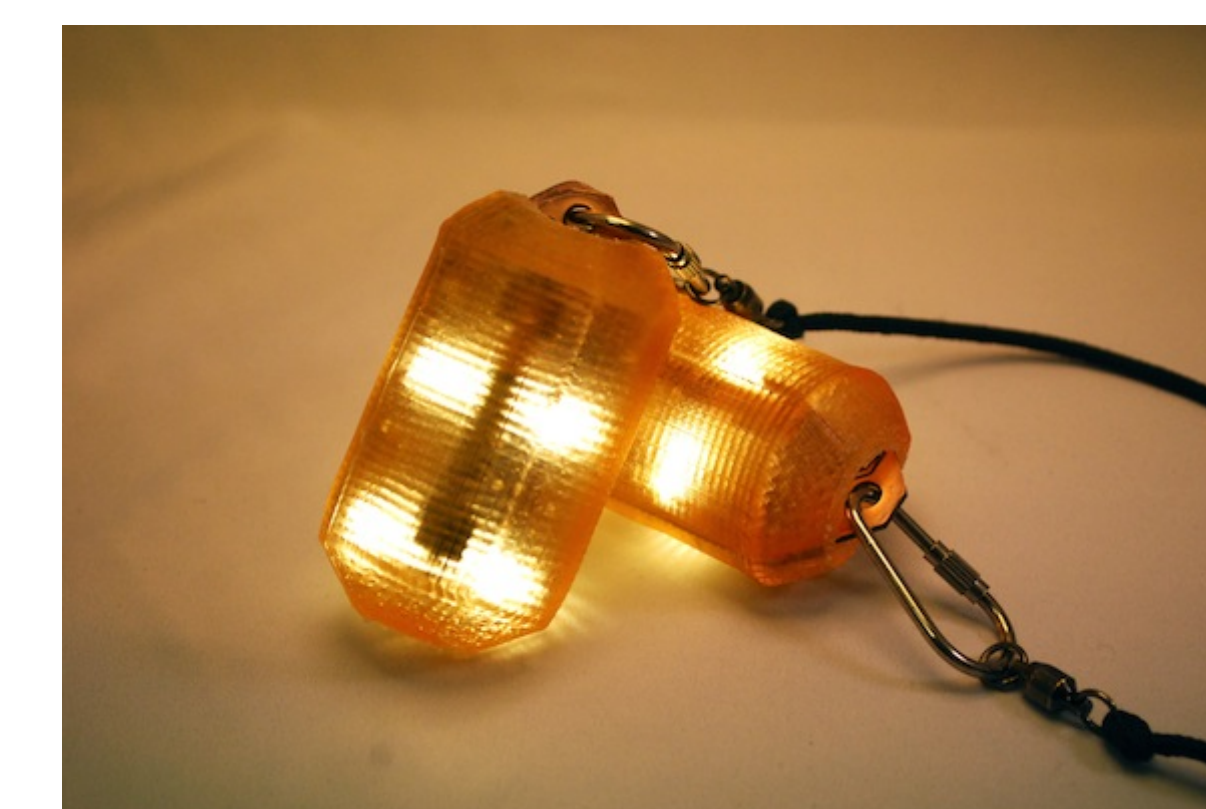
Molds were designed in our own CAD software and manufactured on a Roland Modela mill. Flexible silicone rubber was cast to create protective covers for glowing toys.
