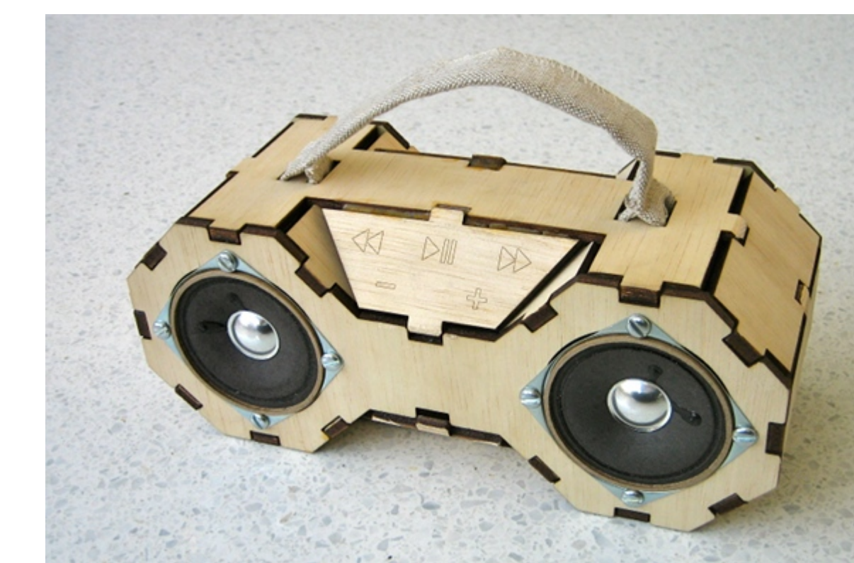
This boombox case was designed as a parametric press-fit construction kit in our own CAD software and fabricated on a laser cutter.
